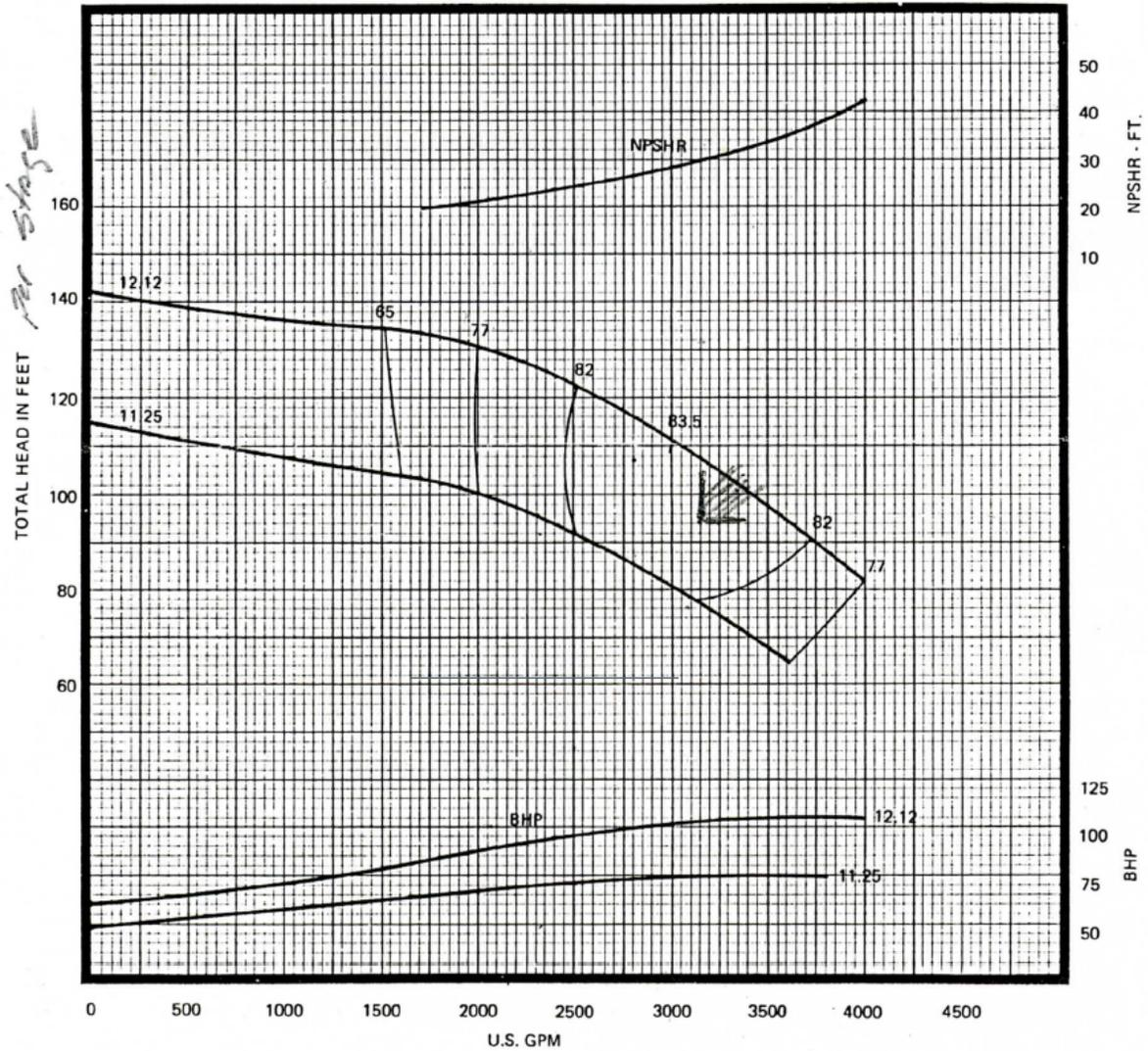
Figure 23 Manufacturer's High Service Pump #1 Curve
