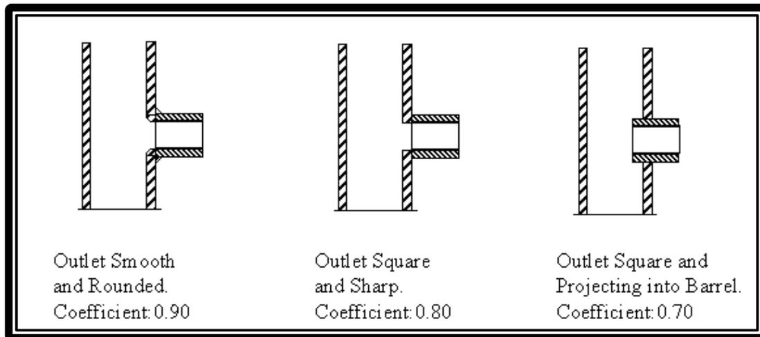
**Figure 27 Hydrant Nozzle Discharge Coefficients**
