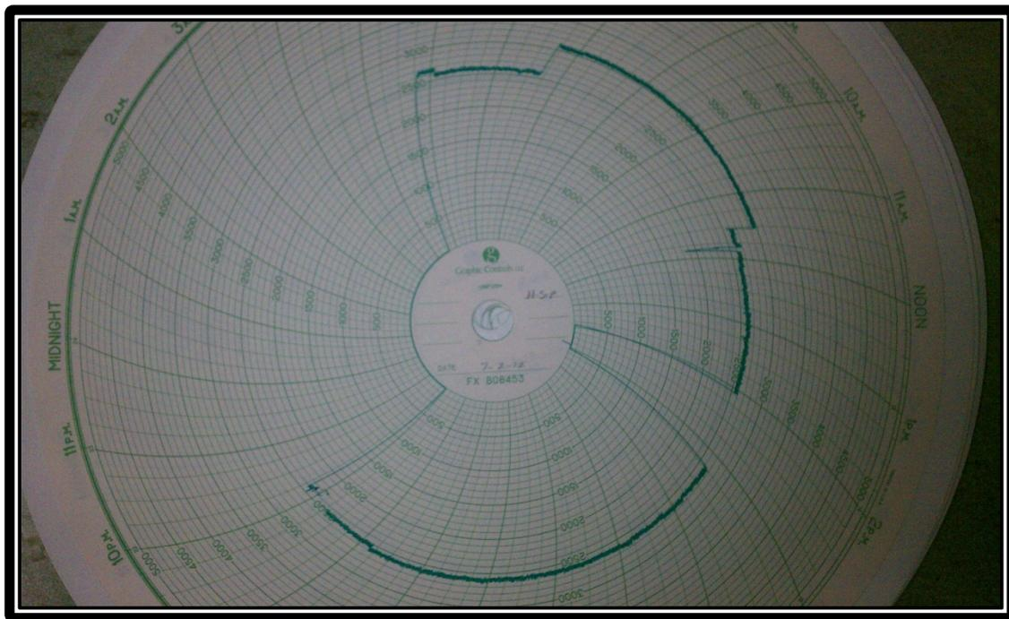
**Figure 14 Example Dial Recorder - Pump Flow on 7/2/2012**
