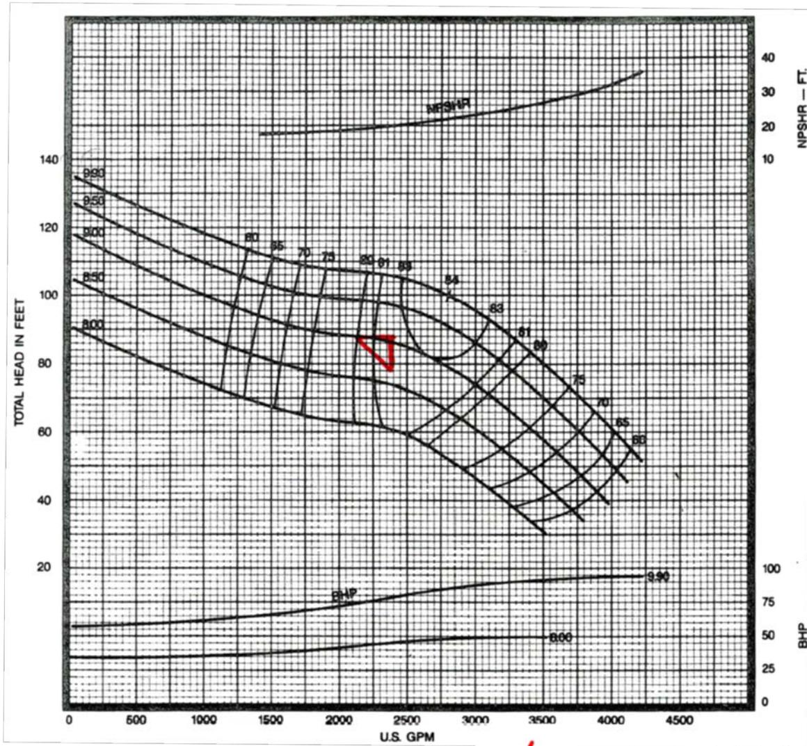
Figure 24 Manufacturer's High Service Pump #2 Curve
