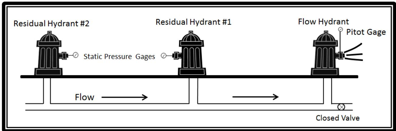
**Figure 11 C-Factor Test Setup**
