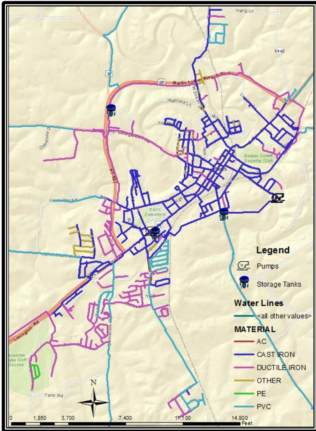
Figure 9 Pipe Materials in Water Distribution System
