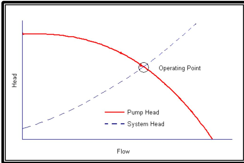
**Figure 19 System Curve and Pump Curve**
