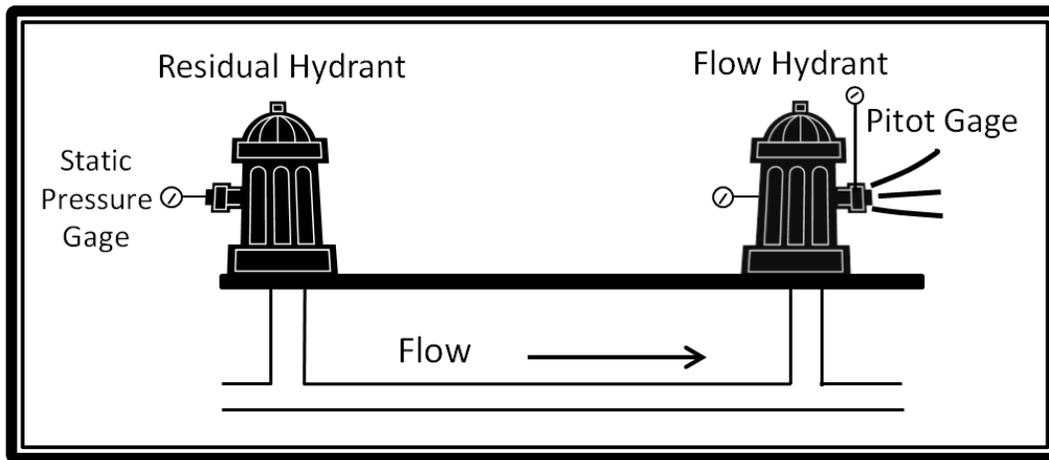
**Figure 13 Fire Flow Test Setup**
