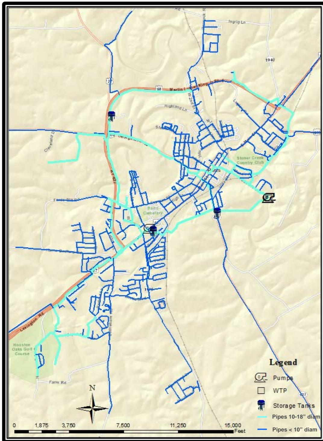
Figure 7 Schematic of Paris Water Distribution System
