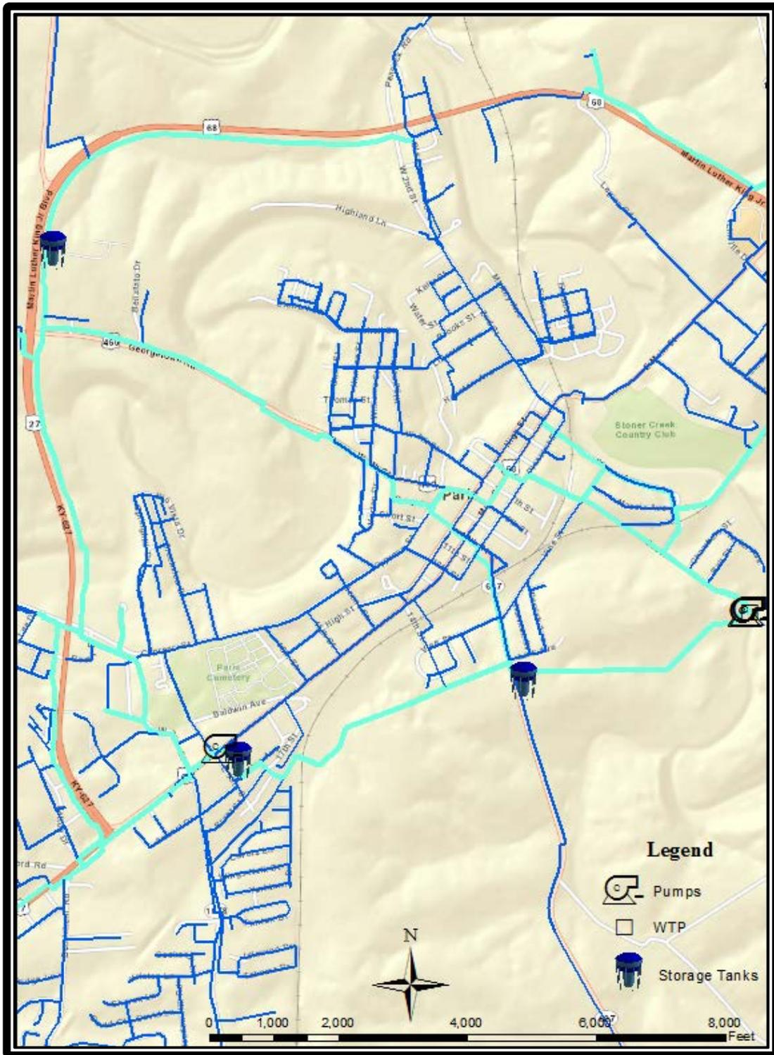
Figure 8 Components of Paris Water Distribution System
